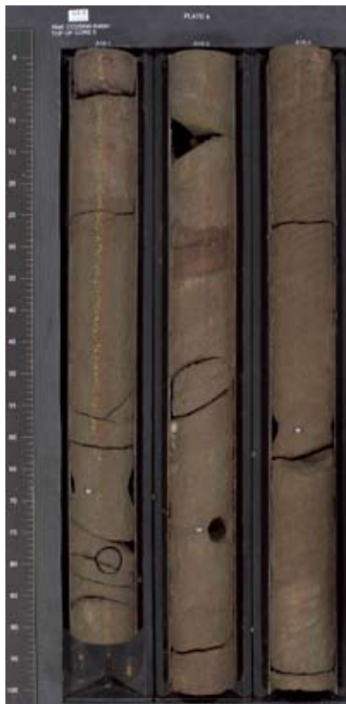
Figure 6. Core image of reservoir sandstone showing cross-bedding.
