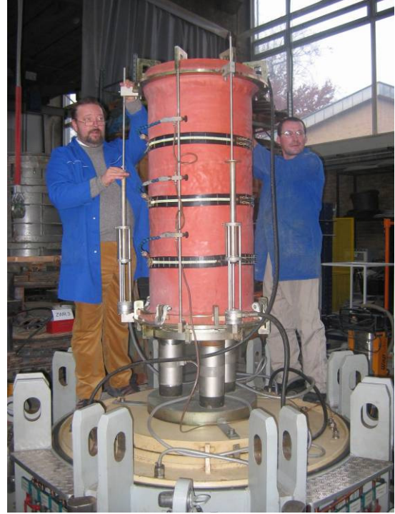
Fig. 2b: Installation of 550 mm specimen in the large triaxial cell
