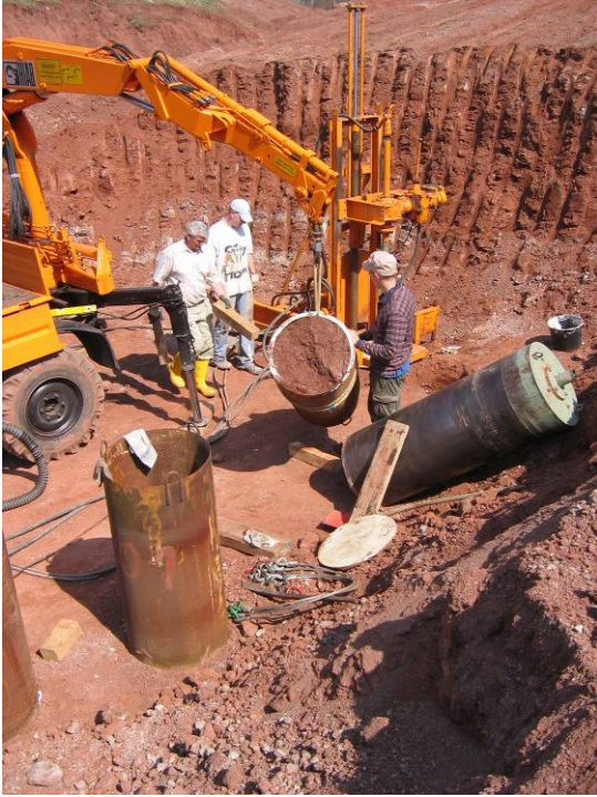
Fig. 2a: Sampling of 550 mm cores in Zaisersweiher
