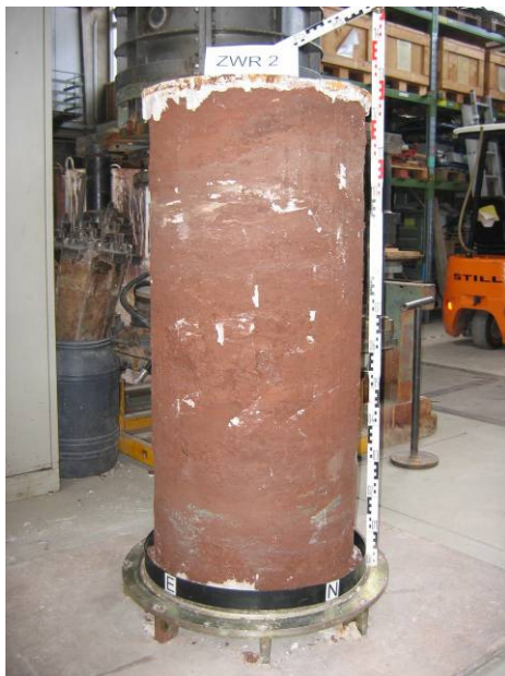
Fig. 5a: Large sample from Keuper clay before triaxial test
