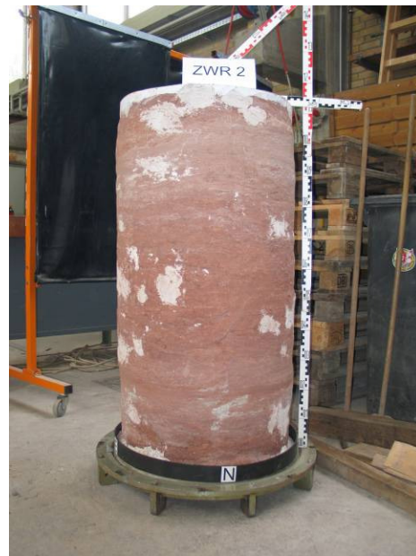
Fig. 5b: Large sample from Keuper clay after triaxial test
