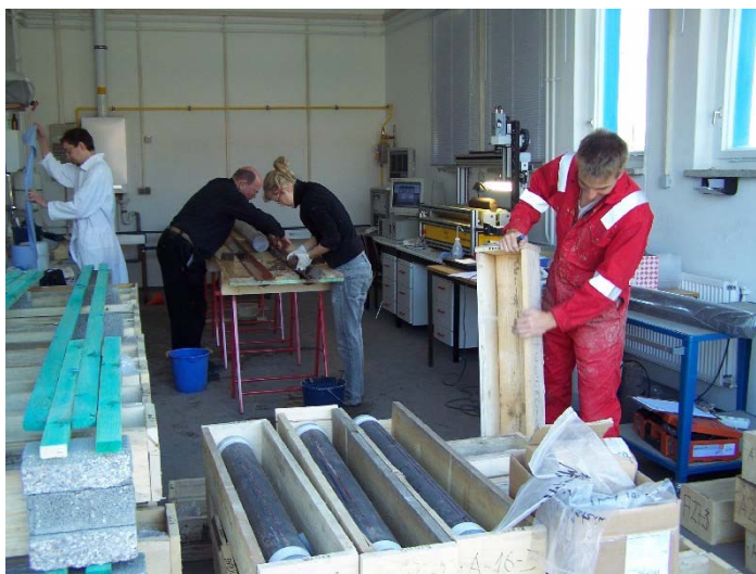
Fig 6 Cores being packed for shipping to the laboratory for further investigation
